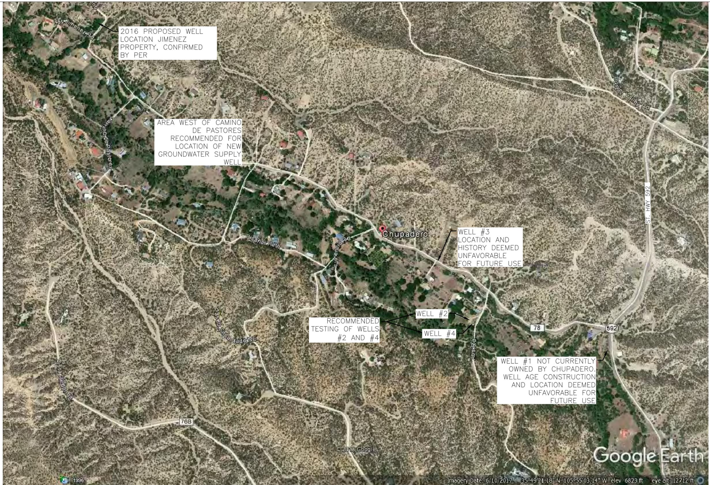
FIGURE 4 – GROUNDWATER SUPPLY WELLS ALTERNATIVE
